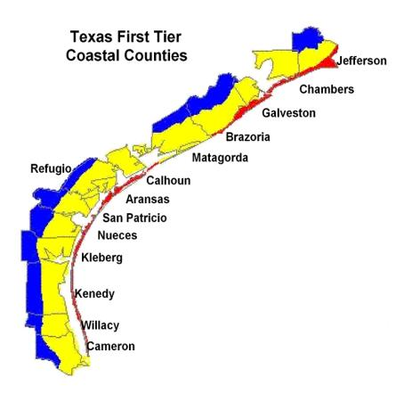
The Seaward construction standard is the strongest and is currently designed to withstand gusts of up to 130 mph. The current Inland I standard is designed to withstand gusts of up to 120 mph and the current Inland II standard is designed to withstand gusts of up to 110 mph. The relative strength of building codes has increased over the years since the first certifications were required in 1988.
