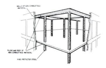
6. Reinforced Concrete Frame (Fire Resistive ISO 6): Risk with this type of construction have structural floors and roof and their supports that are of material such as precast or pouredin-place reinforced construction.
