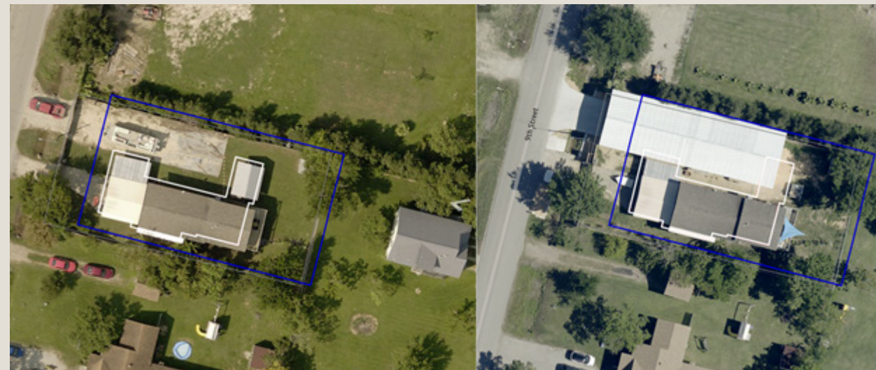
Risk Visualization: TWIA partners with a third party to provide aerial imagery for the Association's coverage territory. The high-resolution imagery -- combined with patented technology for 3D aerial roof measurements -- captured on annual flyovers allows TWIA to remotely inspect a property to determine the accuracy of rating information, discover unrepaired damage, or identify any conditions that may affect the insurability of a property. The example shows a before (left) and after (right) view on two different aerial inspection flyovers of the same property. The white outline details what was detected in the prior year and the blue outline defines the parcel of land.
